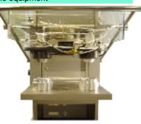
Safe, two handed control system where both hands must be engaged simultaneously
