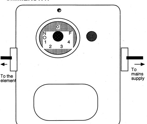
A Simmerstat is a heat control mechanism that can be used in conjunction with either a Little Champion or Medium Champion Pie Machine. Please remember it is not a thermostat. That is to sav it does not maintain the die at anv specific temperature.\_The numbers on the dial give an indication of the length of time that current is supplied to the electric element and hence heating the die.
