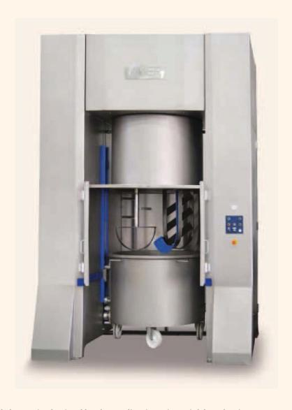
The airtight bowl closure is obtained by the application of special, long lasting gaskets, thus allowing under pressure mixing with extremely filtered, clean air, in observance of sanitation international norms.
