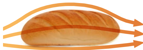
Figure 2: air flows of a Wide Flow double duct system, which allows to generate an enveloping air flow over the product.
