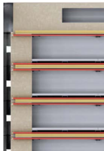
Insulation between chambers
