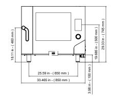
\* Oven must be installed a minimum of 19.7" (500 mm) from any significant source of heat and/or grease (for example: fryers, burners, kettles, open flames, etc.)
