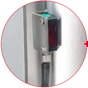
Object detection sensor in the rinsing zone stops rinsing in the absence of items
