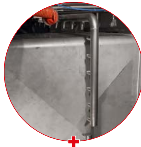
Blow-off nozzles for IBC container exterior drying
