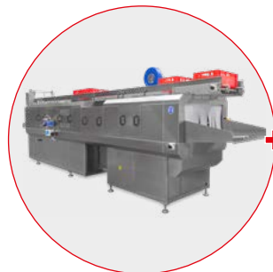
One-man operation: Conveyor on top of the washer
